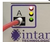
Fig. 26: Third (red) LED light above the yellow and green lights is lit after opening Intan software.
