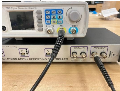
Fig. 9: "Output" BNC of the function generator (left) connected to the "Analog In 1" BNC contact in the Intan controller (right).
