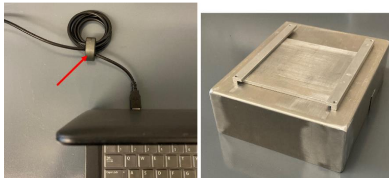
Fig. 12: Ferrite choke on USB cable and EMI shielding cover for the interface board.
