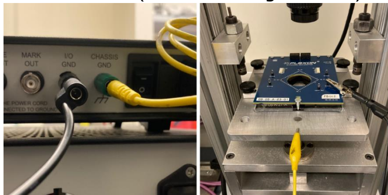
Fig. 11: Connections of the I/O and chassis ground ports on the back of the Intan.
