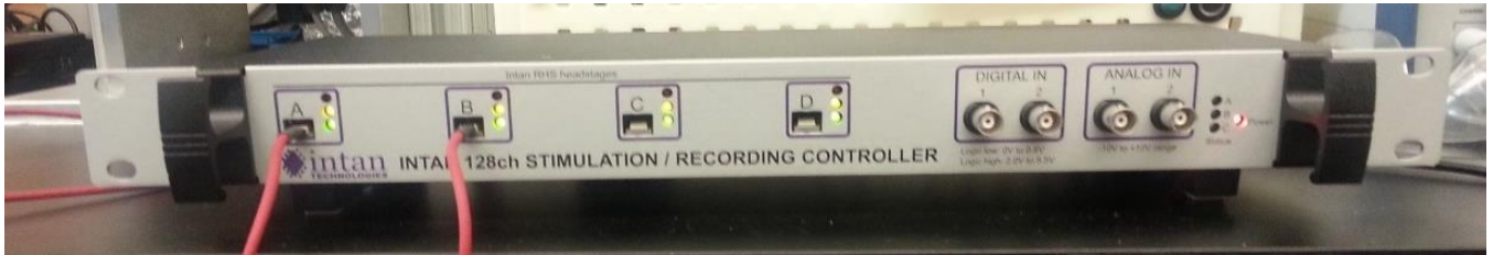
Fig. 8: Recording/stimulation controller with SPI cables connected to Port A and Port B.
