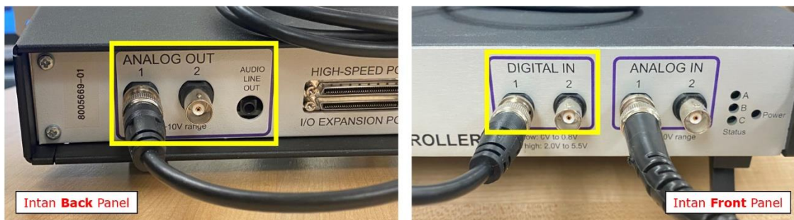
Fig. 90: "Analog Out 1" connected to "Digital In 1" on Intan controller.
