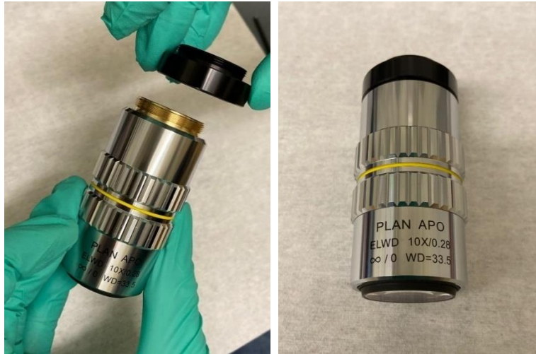
Fig. 118: Attaching the objective coupler to the objective.
