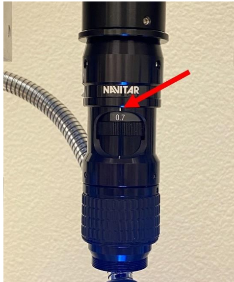
Fig. 70: Camera lens magnification set to smallest value of 0.7×.
