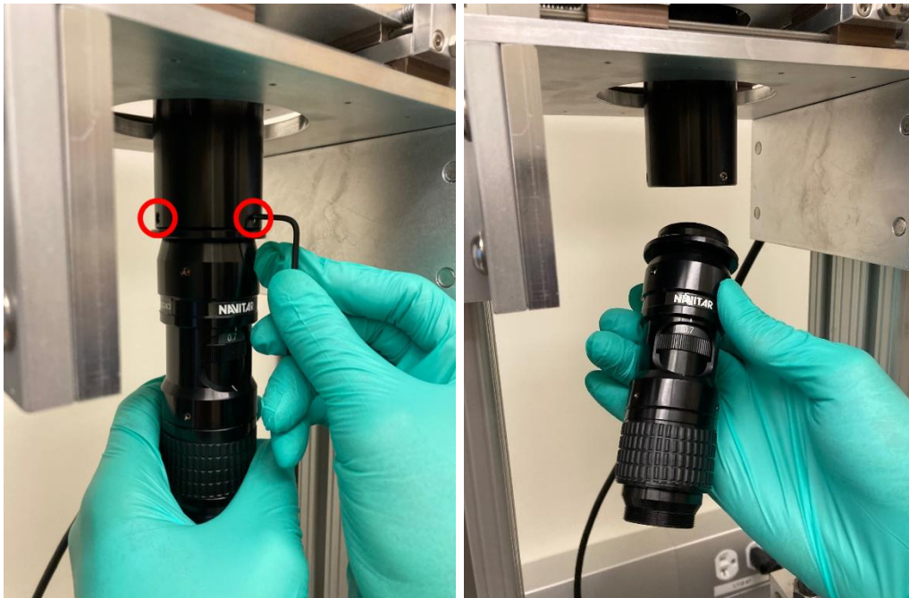
Fig. 115: Removing the zoom lens from the adapter tube.
