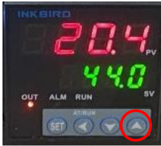
Figure 14. Press the “up” arrow once to enter temperature setting mode.
