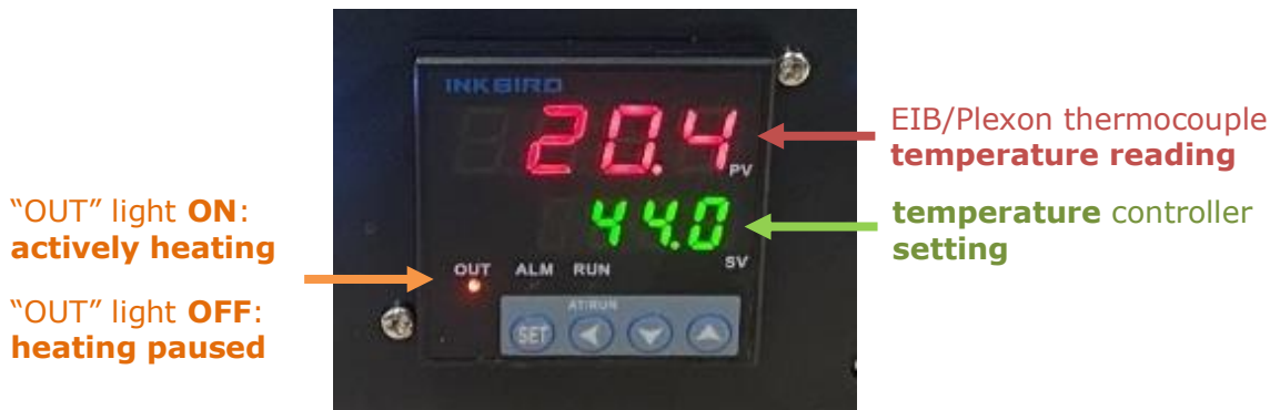
Figure 13. Temperature controller screen with labeled values.
