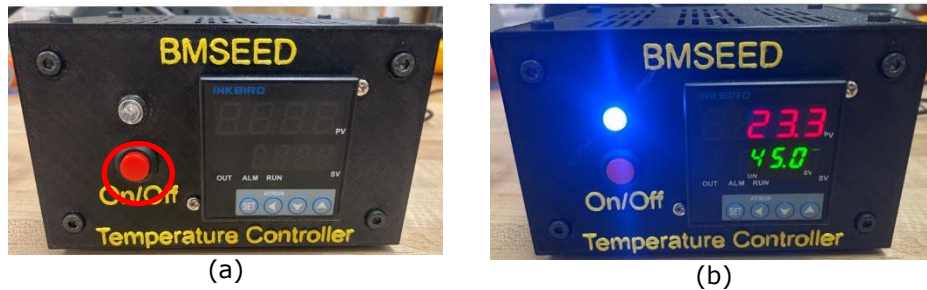
Figure 12. a) front panel of temperature controller with on/off switch labelled "ON/OFF". b) temperature controller turned on after pressing the on/off button.
