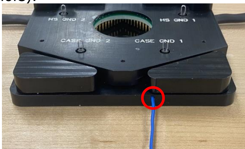
Figure 10. Thermocouple sensor end inserted into hole on bottom plate of EIB
