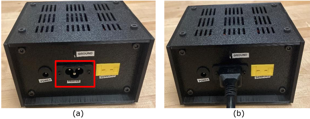
Figure 8. a) backside of temperature controller box with heating resistor connector in the center, labeled "HEATER". b) heating resistor cable plugged into temperature controller box.
